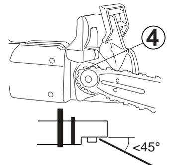
5. Seat the guide bar tensioner pin in its hole in the guide bar.
