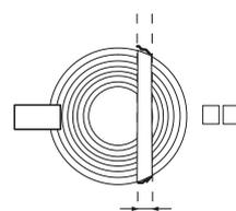
When complete, the FELLING CUT must be parallel to the notch and leave a strip of HINGE WOOD at least 1/10 the diameter of the tree.
