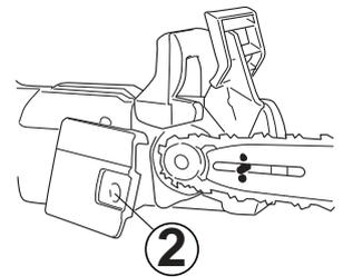
3. Fit the chain around guide bar nose with the top cutters facing forwards.
