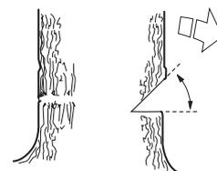
The line defined by the inside angle of the notch must be precisely horizontal and at a precise right angle to the direction of fall.
