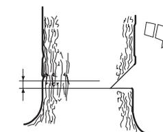
Place the FELLING CUT approximately 3-5 cm (1 1/2 - 2") above the BOTTOM NOTCH CUT.
