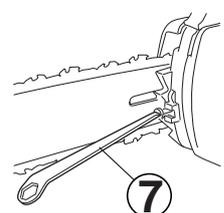
8. The chain is correctly tensioned when the slack on the bottom of the bar is gone, yet the chain is still easily pulled around by hand.
