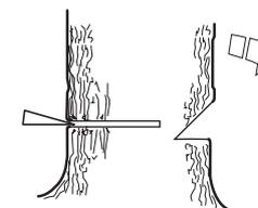
Cut at full motor speed, feeding the saw slowly into the tree. Watch out for tree movement opposite to the intended direction of fall. Insert a WEDGE or FELLING BAR in the FELLING CUT as soon as the depth of the cut permits.
