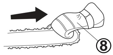
9. Tighten the mounting nut with the combination tool while holding the tip of the guide bar up.
