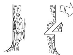
Notch depth should be around 1/4 of the diameter of the tree and the angle should be around 45°.
