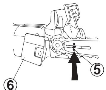
6. Replace the chain drive cover and screw the mounting nut hand tight.
