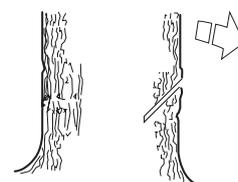
Next do the BOTTOM NOTCH CUT, ensuring that it meets the bottom of the TOP NOTCH CUT precisely.
