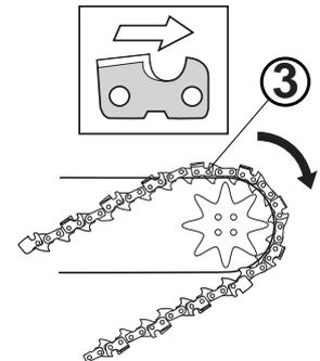
4. Holding the chain over the guide bar nose, position the back end of the guide bar against the drive sprocket at a 45° angle to the power head. Pass the free end of the chain around the drive sprocket, swing the guide bar into place over the mounting bolt and against the power head, and guide the chain into the guide bar groove.
