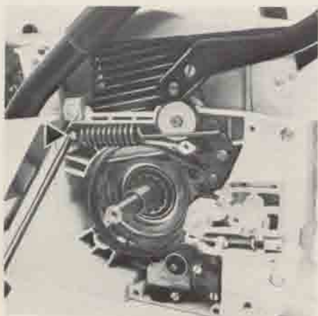
Unhooking the extension spring
