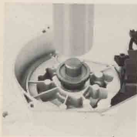
Forcing out the ignition end ball bearing.
