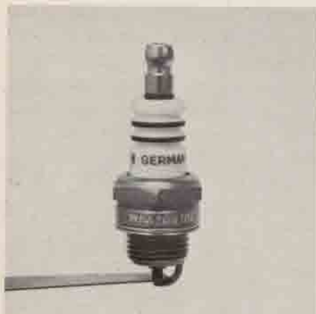
Checking the spark gap with the feeler gage
