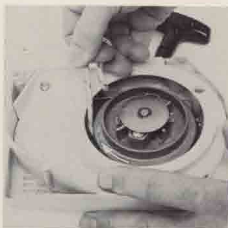
Tensioning the rewind spring
