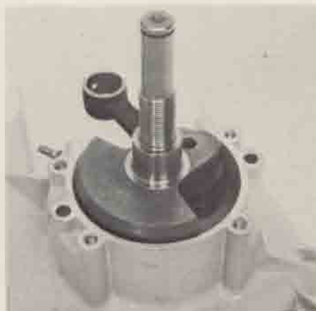
Crankshaft slid in up to the crank check
