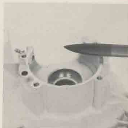
Bottom: Circlip installed
