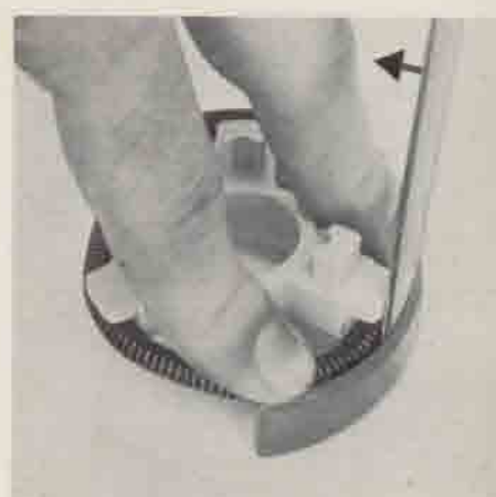
Levering the driver in place
