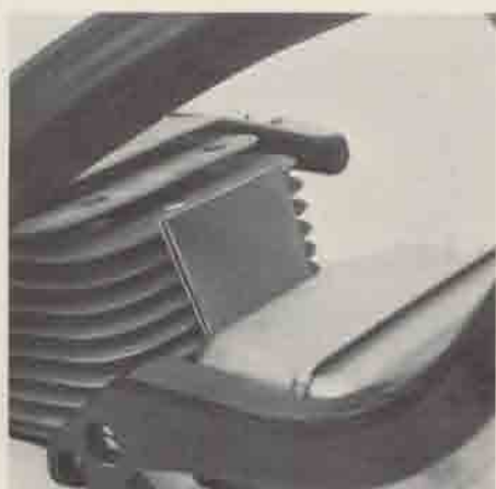
Seal plate installed
