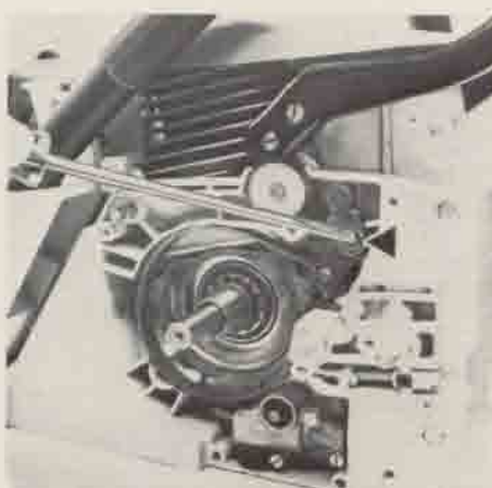
Middle and bottom: Unscrewing the hand guard
