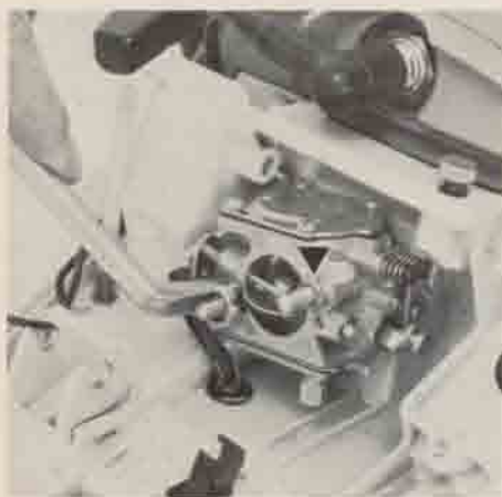
Removing the carburetor
