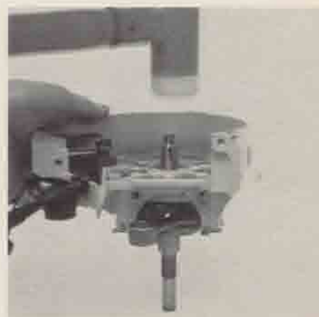
Bottom: Driving out the shaft seals
