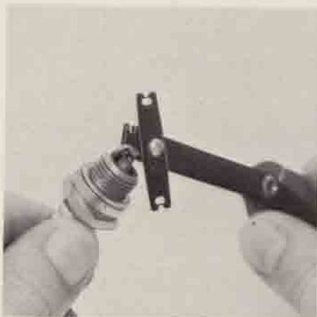
Adjusting the electrode gap with the Bosch spark plug gage
